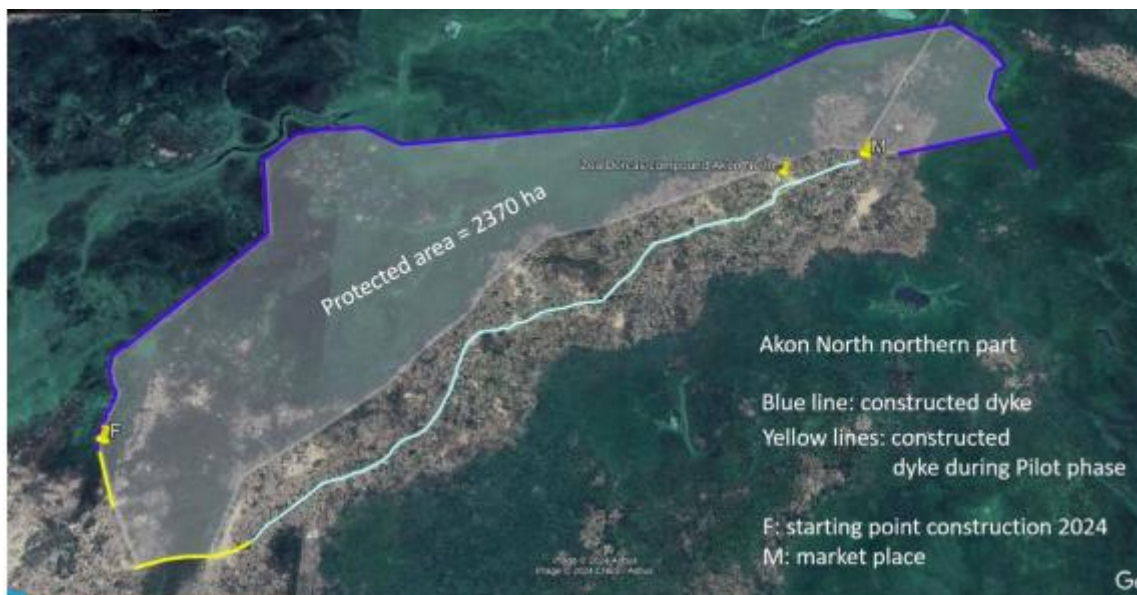
Figure 4 Phase 1 Dike to be repaired, reinforced and topped-up to the safety level standard (18km)
