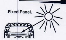
Place the radio in the sun so that the sunlight falls onto the solar panel on the top/back of the radio.
