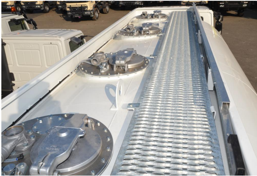
Open mesh walkway on the right-hand side of the manhole cover and collapsible handrail made of aluminum, operated manually, fixed as safety barrier, along the dome-pan. Operation of handrail manual, next to access ladder.
