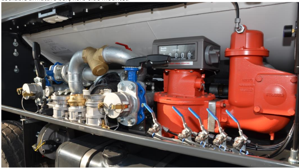
Lockable cabinet with discharge outlets. Pneumatic operations. Metering system.
