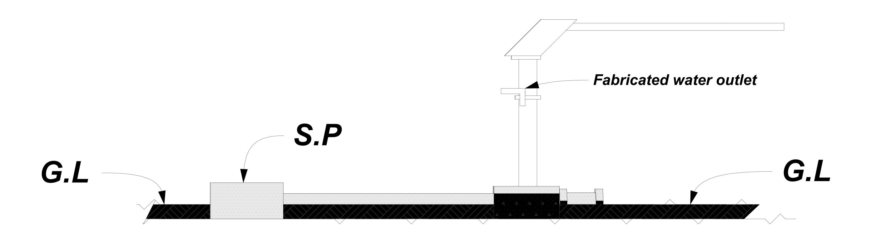
The design of the handpumd is to be according to the industrial standards statated only a modification is to be made on the water outlet to enable PWD access water easily
