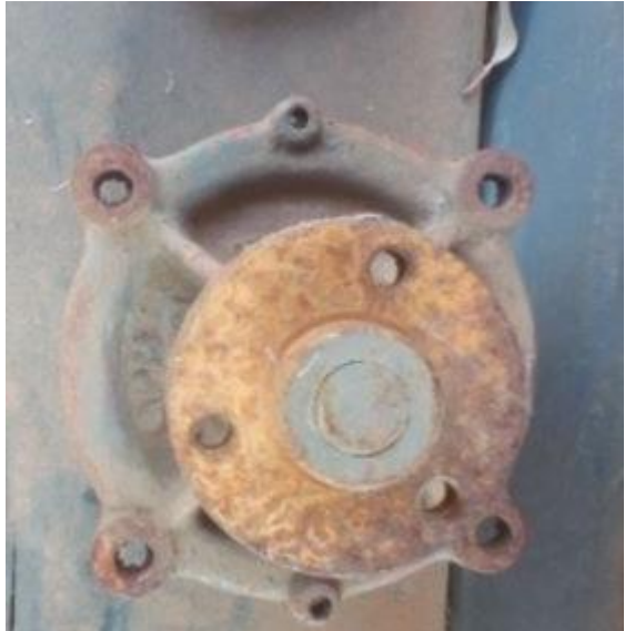
Pump Bucket seal (old model) XAS 186 model, use for compressor machine seen on left side
